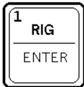
Used to by-pass permanently the lockout while rigging the crane. The Enter function is used to confirm other actions.
