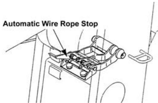
This device prevents the wire rope on the drum from slackening when the hook makes an abrupt stop or when the hook/load is lowered to the ground.
