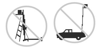
Do not use the machine on a moving or mobile surface or vehicle.
