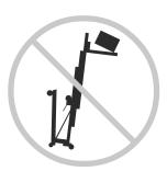
Do not remove the leg retainer pins while the machine is loaded and/or raised.
