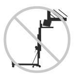
Use good judgement and planning when transportig the machine on an incline or slope.
