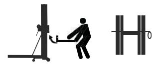
Adjust the forks to the desired width.
