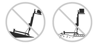
Prior to use, check the work area for drop-offs, holes, bumps, debris, unstable or slippery surfaces or other possible hazardous conditons. Do not raise the load unless the load handling atachment is properly secured to the machine.
