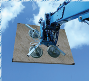
Lift a wide range of materials by changing the suction cups
