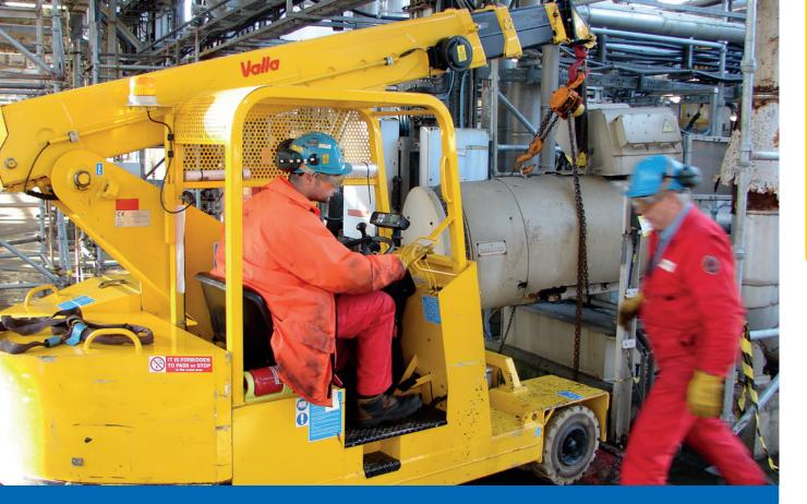
The Valla 50E combines a 5,000kg lifting capacity with precise load control and fume-free operation
