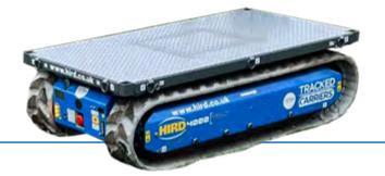
The new 4000 PRO from Tracked Carriers offers an unrivalled method of transporting heavy goods through confined spaces. At only 1m wide, the 4000 PRO has a maximum capacity of 4,000kg and can climb gradients up to 45° with a reduced load.
