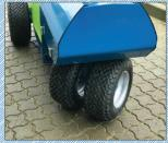
Winlet 400 TL is equipped with extra wide steering traction wheels provide greater stability and the capability to manoeuvre outdoors.
