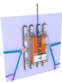
The falling safety devices are implemented by means of lifting straps with hooks, which must be hooked to the suction pad. During use the following shall be observed.
