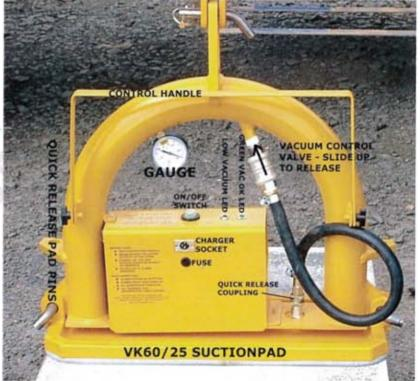
LOAD IS CORRECTLY DIVIDED OVER THE SUCTION PAD - THE UNIT SHOULD BE CENTRED ON PANEL TO BE LIFTED. UNIT IS THEN LOWERED ONTO PANEL ENSURING THAT THE PAD DOES NOT OVERLAP MATERIAL BEING LIFTED AND THAT IT IS PRESSED AGAINST PANEL.
