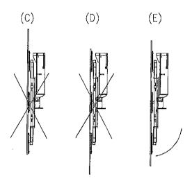
Check that all suckers on the surface are clean and have full contact and, if necessary, press on or align a sucker that is not making contact until it is in the correct position. If this is not done, a vacuum cannot build up and the DSMH4-24V can therefore not lift the material. Set the suction/release valves to the suction position using the remote control.
