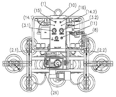
Switch the machine to ON using the on/off switch (10). The pumps must start up if the vacuum is insufficient. The Pump indicator light (16 yellow) indicates that the pumps are ready for operation. If this is not the case, working with the DSMH2-12V is not permitted (see Troubleshooting).
