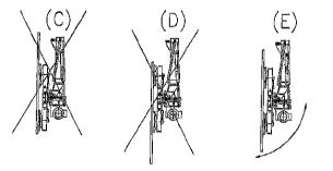
Check that all suckers on the surface are clean and have full contact and, if necessary, press on or align a sucker that is not making contact until it is in the correct position. If this is not done, a vacuum cannot build up and the DSMH2-12V can therefore not lift the material. Set the two suction/release valves (2.1 and 2.2) to SUCTION using the remote control.
