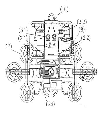
The individual suckers (7) must be connected to the vacuum reserve tanks by opening the blocking valves (26).
