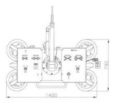
In particular, the device consists of a rectangular tube frame with suspension eye, the basic frame. A second rectangular tube frame is connected to this basic frame first via a swivelling joint and then via a rotating joint. This frame is the carrier frame which simultaneously forms the vacuum reserve tank and holds the vacuum pump, the battery loading device, and the batteries.
