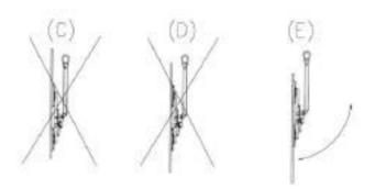
Check whether all suction cups on the surface are clean and have full contact, and if necessary press on or align a suction cup that is not making contact until it is in the correct position. If this is not done, no vacuum can build up and the DSZ2-12V cannot carry out any lifting of materials.
