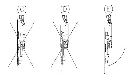
Check that all suckers on the surface are clean and have full contact and, if necessary, press on or align a sucker that is not making contact until it is in the correct position. If this is not done, a vacuum cannot build up and the DSZ2-12V can therefore not lift the material. Set the two manual suction/release valves (2.1 and 2.2) to SUCTION.
