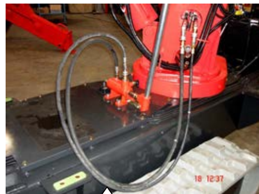
Illustration 5 showing crane ready for emergency winching
