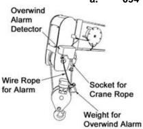
Refer to the figure on the left for crane rope routing and location of the weight for the overwind alarm
