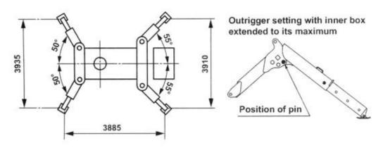
Example: Outrigger setting to a distance below maximum (Figure shows they are set to minimum extension).
