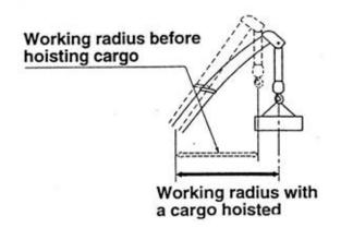
The working Range chart does not take into account of movement due to boom deflection.
