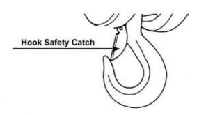
The hook safety catch is used to retain lifting accessories in the correct place on the hook
