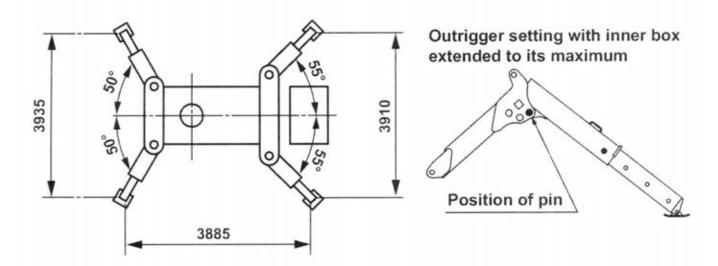
Example: Outrigger setting to a distance below maximum (Figure shows they are set to minimum extension).
