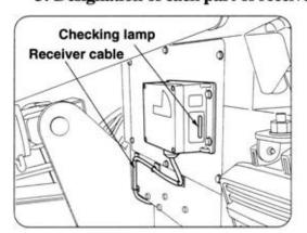
\*Receiving antenna is built in the receiver.
