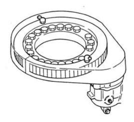
If the slew ring makes an unusual noise when operating or crawling, or excessive movement is observed when operating the crane, or if a gap is observed on the mounting surface, contact your UNIC service agent immediately for inspection and/or repair
