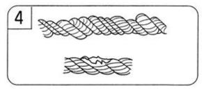
4. A rope that has become deformed or excessively corroded
