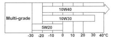
The selection of the correct engine oil is vital to the engine. Choosing the wrong oil or neglecting an oil change can result in severe damage to the engine.
