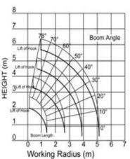
Note: The chart shows the data when the crane is operated with no load and shift due to deflection is not considered
