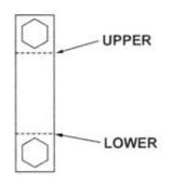
The proper level is between the 'UPPER' and 'LOWER' limits illustrated left
