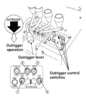
There are four switches and one lever used for outrigger.
