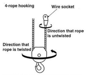
(Note) Rotate wire socket to the direction opposite to wire ropes have been twisted.
