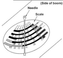
The indicator reads the rated load corresponding to the boom extension and angle. This is the maximum load that can be lifted at that point
