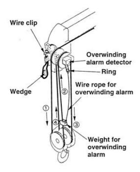
Refer to the figure on the left to follow the routing of the rope and where the weight for the overwind alarm is to be mounted
