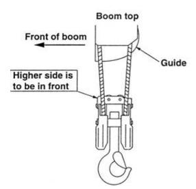
Refer to the figure on the left for the correct way to attach the hook block
