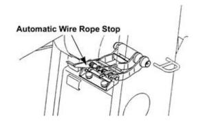
This device prevents the wire rope on the drum from slackening when the hook makes an abrupt stop or when the hook/load is lowered to the ground.
