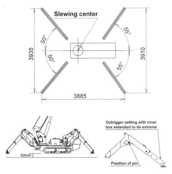
The figure above shows the outriggers extended to their extremes. Carry out operations by first ensuring the outriggers are on firm, level and uniform ground. This may require the use of timber or steel plates. Extend the outriggers to
