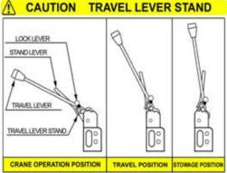
When changing the position of the travel lever stand, always use the stand lever and NOT the travel levers CRANE OPERATION POSITION
