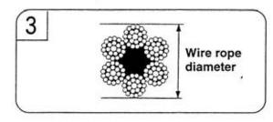
3. A rope whose diameter has decreased by more 7% of the nominal diameter. For example: where a rope of 8mm nominal diameter is used, replace it when any part of the rope is 7.5mm
