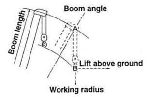
Although Point A and Point B follow the same track along the working radius, due to boom deflection Point A refers to the boom angle and Point B refers to the lift above ground
