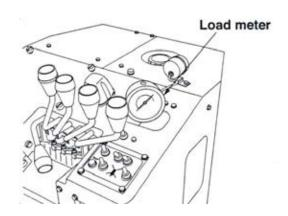
The meter shows the weight of a load being hoisted. Read the scale band corresponding to the number of falls of rope
