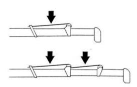
Apply grease to the boom extension ropes once a month, ensuring the boom is fully extended
