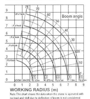
radius, boom angle and lift above ground
