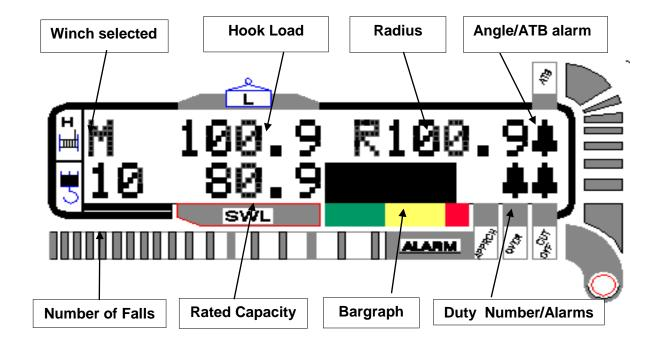
Using button **(#5) DISPLAY** the operator can access other functions of the system like Error report and Diagnostics for maintenance purposes. These functions are displayed for 15 seconds before the system returns to the normal display.
