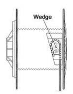
Refer to the figure on the left for correct wedge attachment to the drum
