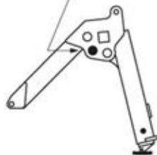
Outrigger setting with inner box extended to its minimum
