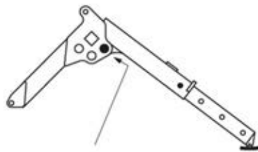
Outrigger setting with inner box extended to its maximum
