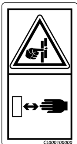
(23) Do not insert fingers into the hole (CL000100000) (4 places)
