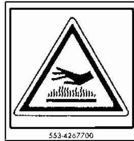
(14) High temperature caution (553-4267700)
