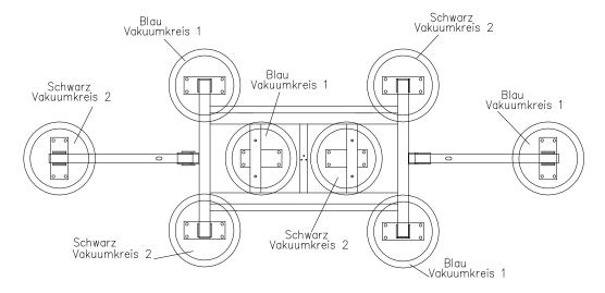
Without extensions, suction pads attached to the vacuum cross arm
