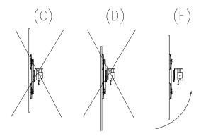
Check that all suckers on the surface are clean and have full contact and, if necessary, press on or align a sucker that is not making contact until it is in the correct position. If this is not done, a vacuum cannot build up and the GA2 can therefore not lift the material. Activate the Suction key.
