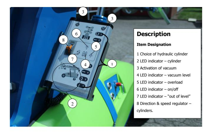
The WinLet 575 is equipped with an operating panel from which all vacuum and hydraulic functions are controlled. The integrated safety functions are:
