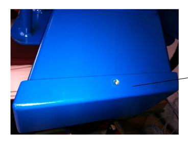
Remove cover to access the grease nipples
